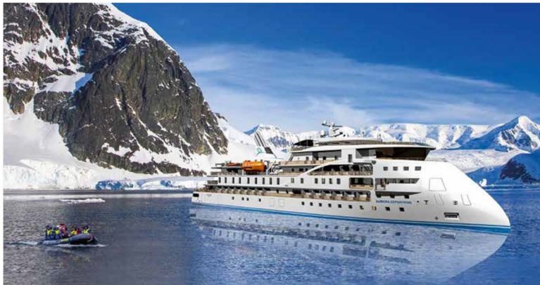
Aurora Expeditions' newbuild will be the first to feature Ulstein Group's X-BOW hull so she can pierce waves with greater stability, increasing passenger comfort
